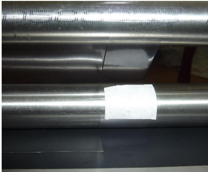
10-Pay attention while pulling the cellophane towards packaging the boxed, don't jerk the film be soft and constant with film movement. The excess will be automatically wrapped on the steel cylinder and it will grow up.
